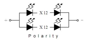
Note: Circuit layout is 12 series and 2 parallels
