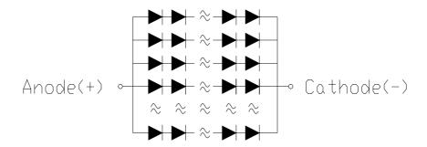
Note: Circuit layout is 12 series and 14 parallels
