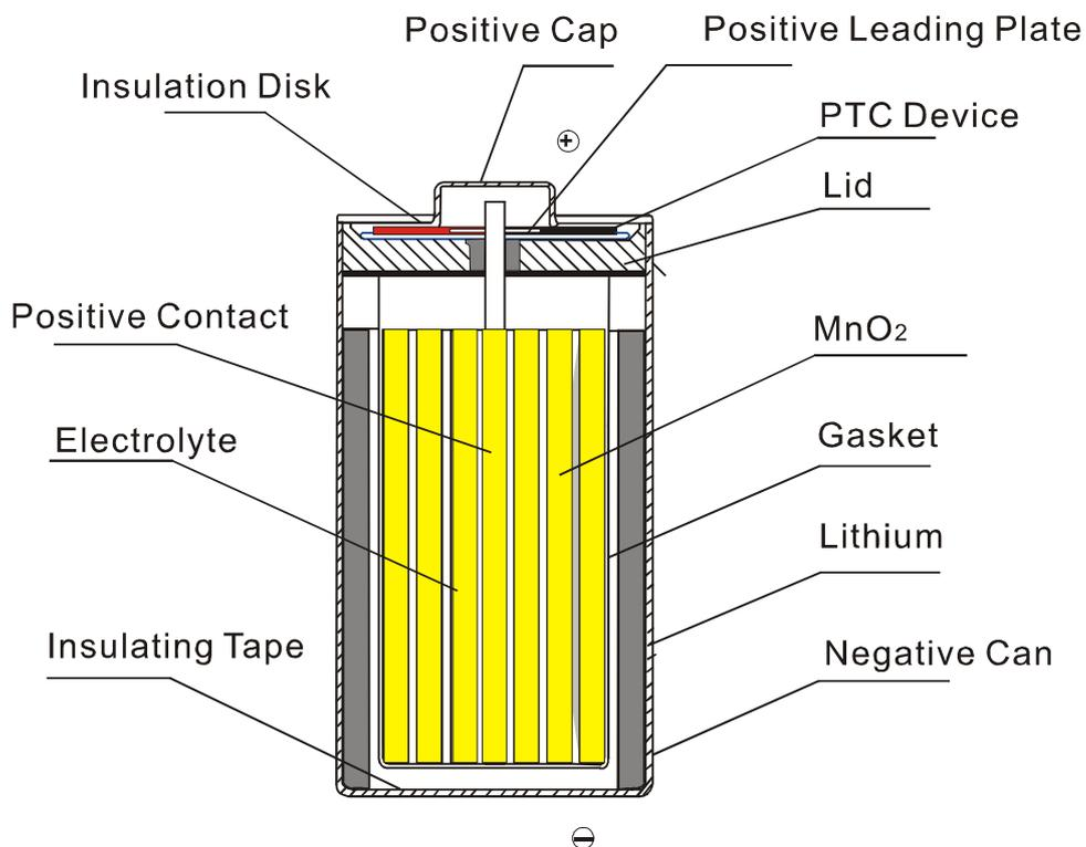
**Spiral structure, laser-sealing**
