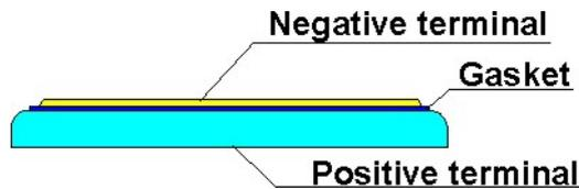
When batteries are overlapped or mixed together in a disorder way, their positive and negative terminals touch each other, causing short circuits.
