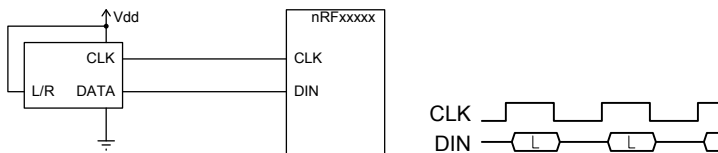
Figure 119: Example of a single PDM microphone, wired as left
