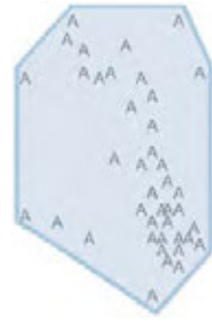
CellLocate server defines area of cell visibility
