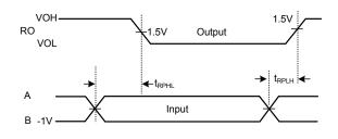
Fig. 9 Receiver Propagation Delays
