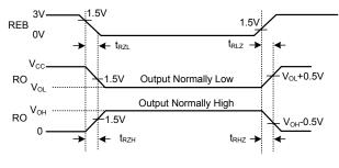
Fig. 10 Receiver Enable and Disable Times
