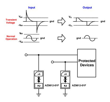
Fig. 1 ESD protection scheme by using AZ9812-01F.
