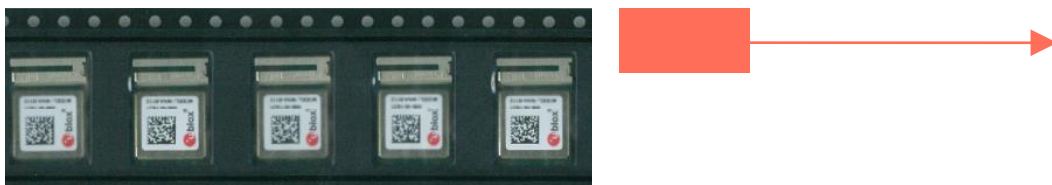
Figure 12: NINA-W102/NINA-W106 module on tape orientation
