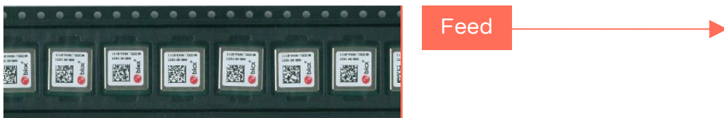
Figure 11: NINA-W101 module on tape orientation
