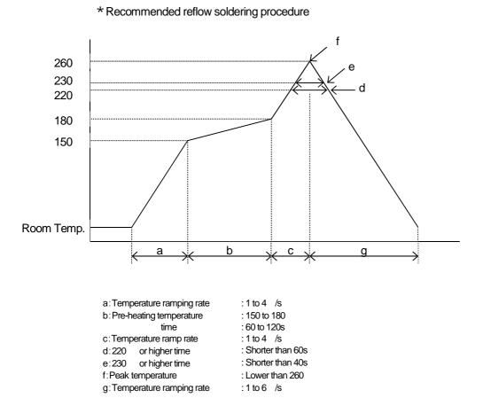
The temperature indicates at the surface of mold package.
