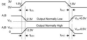
Fig. 8 Transmitter Enable and Disable Times
