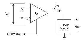
Fig. 6 Receiver Output Short Circuit
