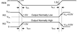
Fig. 9 Receiver Propagation Delays
