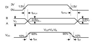
Fig. 7 Transmitter Propagation Delays
