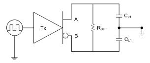
Fig. 2 Transmitter Timing Test Circuit
