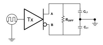
Fig.2 Transmitter timing test circuit
