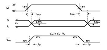
Fig.7 Transmitter Propagation Delays
