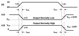
Fig.8 Transmitter Enable and Disable Times
