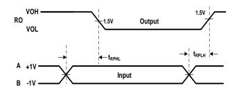
Fig.9 Receiver Propagation Delays
