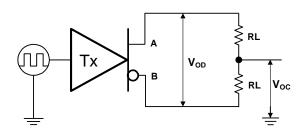
Fig.1 Transmitter DC test circuit
