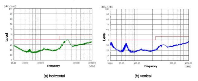
Figure 2-6 EMI result on equivalent VCCI CLASS-B 3m
