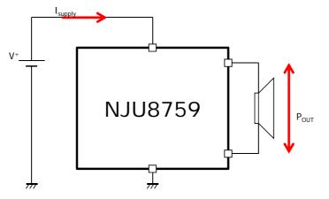
Figure 2-3 a power dissipation model
