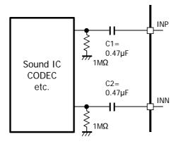
Figure 2-2 How to prevent floating input pins
