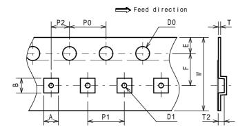
SYMBOL DIMENSION REMARKS A  $1.55 \pm 0.05$ BOTTOM DIMENSION BOTTOM DIMENSION В  $1.55 \pm 0.05$ DO 1.5<sup>+0.1</sup> D1  $0.5 \pm 0.1$ Е  $1.75 \pm 0.1$ F  $3.5 \pm 0.05$ P0  $4.0 \pm 0.1$ P1  $4.0 \pm 0.1$ P2  $2.0 \pm 0.05$ Т  $0.25 \pm 0.05$ T2  $0.7 \pm 0.05$ W 8.0 +0.3
