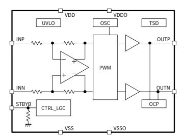
Figure 1-1 the NJU8759 block diagram
