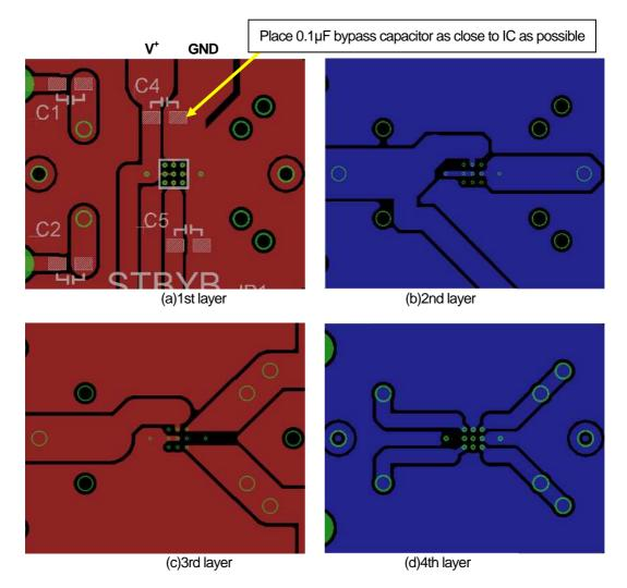
Figure 2-7 an example for 4 layer PCB Layout around the NJU8759
