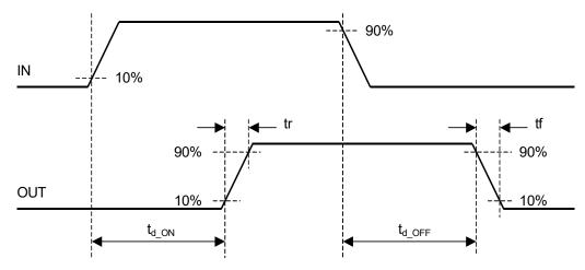
Fig1. Output Rise/Fall Time, Rise/Fall Delay Time
