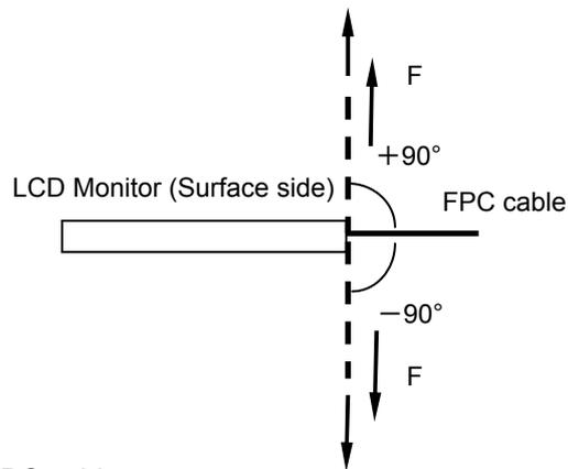
Bend Test Method for FPC cable
