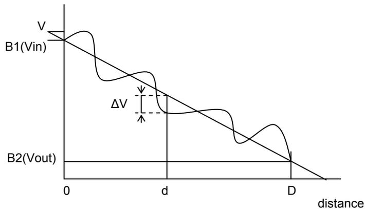
$$LE(\%) = \frac{\Delta V}{(V_{in} - V_{out})} \times 100$$
