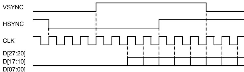
Example 3 : DI4=DI5=1, DI6=0 (CLK is reversed, data is read at the rising edge of CLK.)
