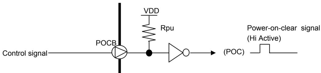
In case of directly controlling POCB terminal, POCB terminal should be set to "Lo" at Power-on. POCB should be changed to "Hi" after VDD is exceeding 2.7V. Serial communication is prohibited while POCB is "Lo".
