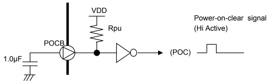
POCB terminal is connected to VDD through the pull-up resistor ( $R_{pu}$ ).
