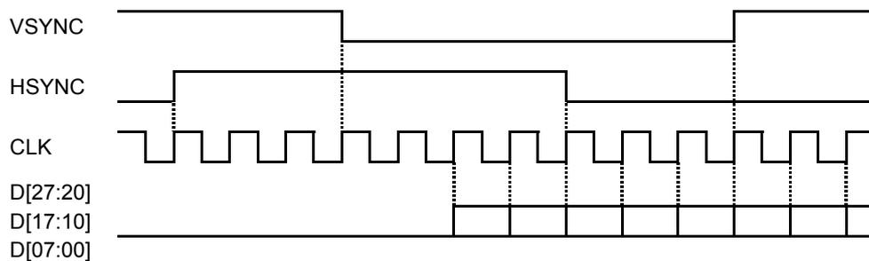
Example 2 : DI4=1, DI5=0, DI6=1 (VSYNC has positive polarity and Hi active)
