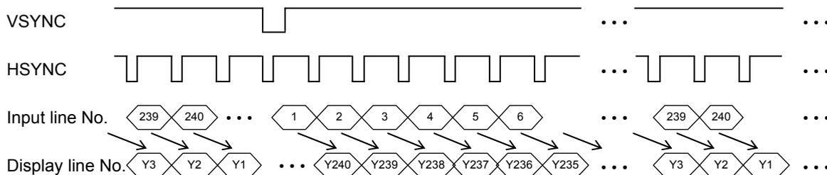
\* Above timing chart shows correlation between input data and pixels in visual way and it is not actual timing chart.
