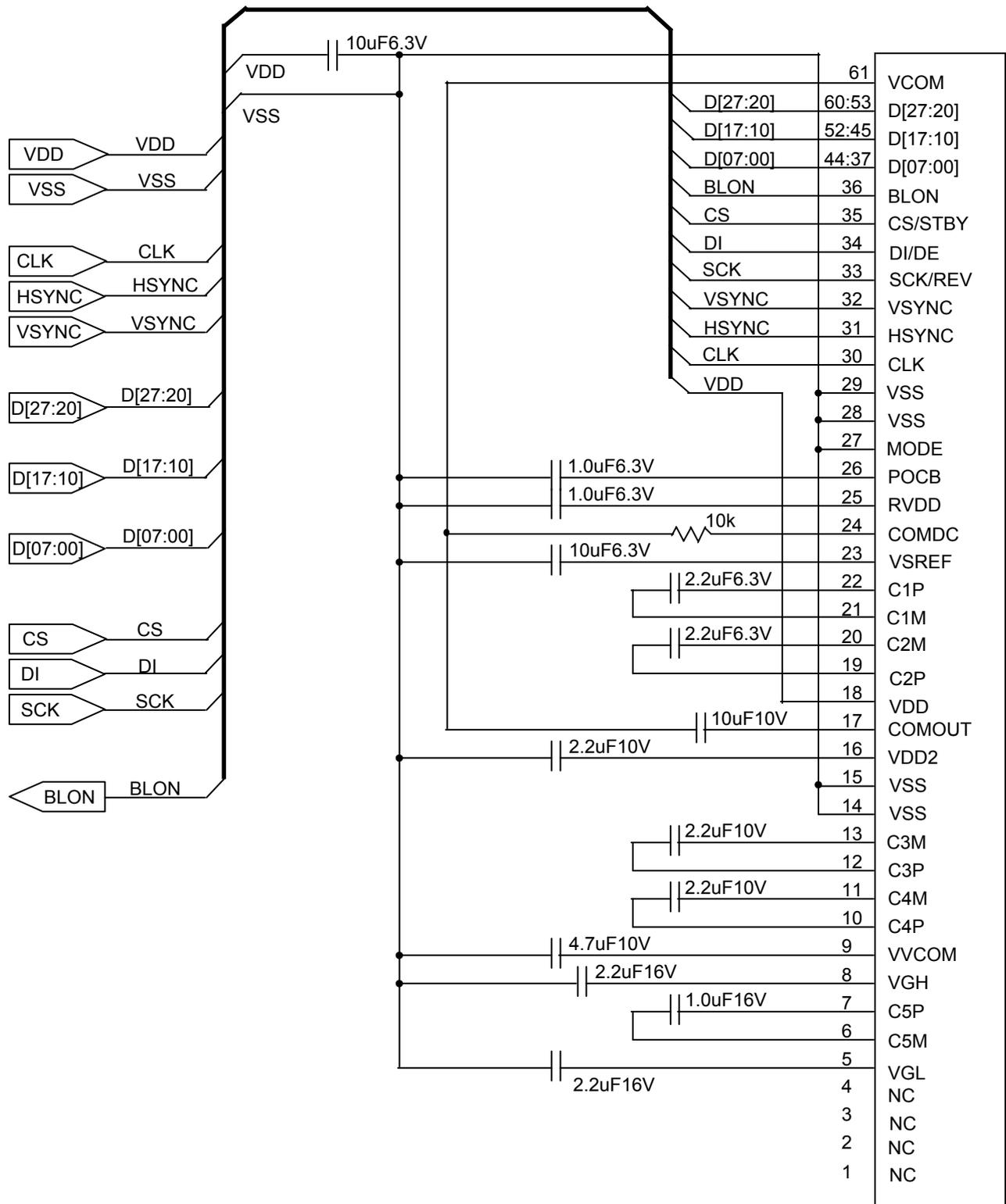
TFT LCD MODULE REFERENCE CIRCUIT
