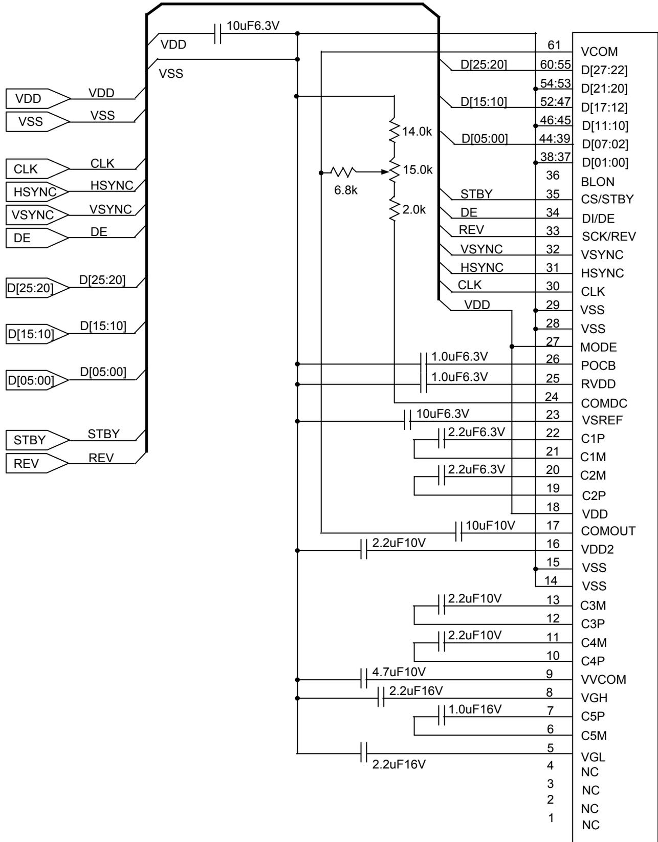
TFT LCD MODULE REFERENCE CIRCUIT
