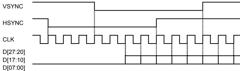
Polarity of each signal can be changed independently by logic of DI4, DI5 and DI6.
