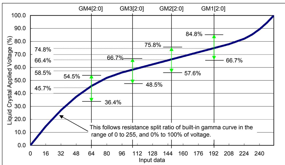
When no correction is made to gamma potential of GM1 to GM4;
