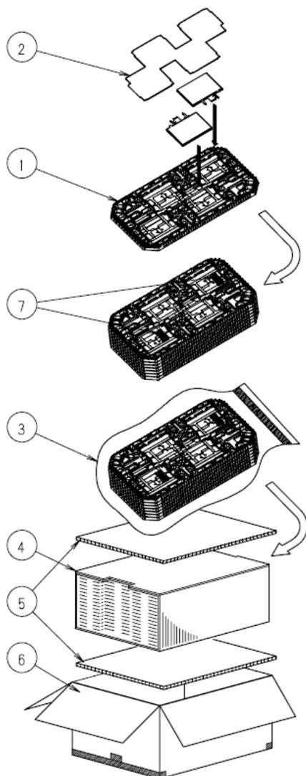
Step 1. Each product is to be placed in one of the cut-outs of the tray with the display surface facing upward.(4products per tray)
