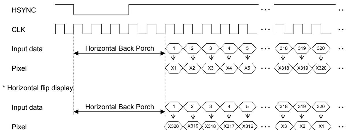
\* Above timing chart shows correlation between input data and pixels in visual way and it is not actual timing chart.
