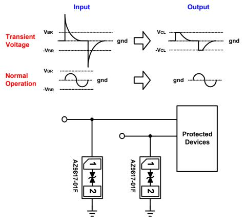
Fig. 1 ESD protection scheme by using AZ9817-01F.
