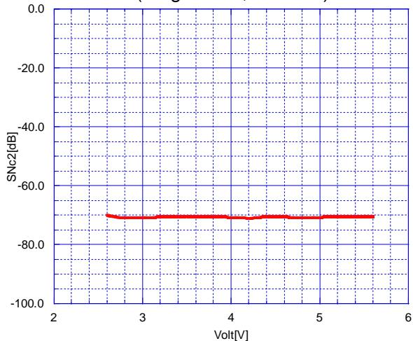
S/N Ratio vs. Operating Voltage
