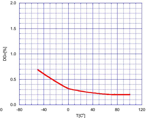
Differential Phase(V mode) vs. Temperature
