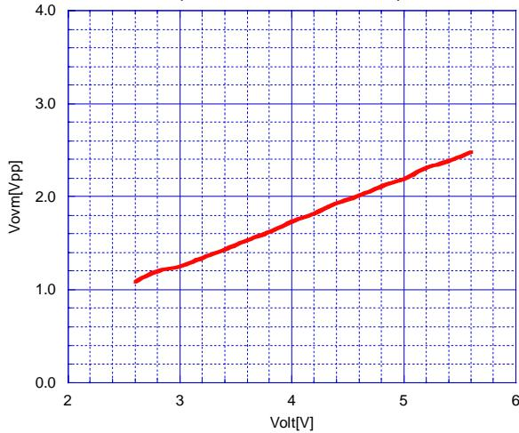
Differential Gain vs. Operating Voltage
