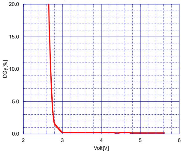
Differential Phase vs. Operating Voltage
