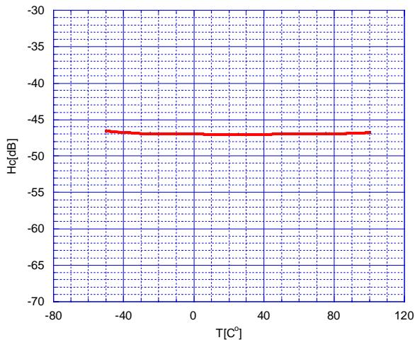
2<sup>nd</sup> Distortion vs. Temperature
