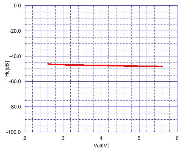
2<sup>nd</sup> Distortion vs. Operating Voltage
