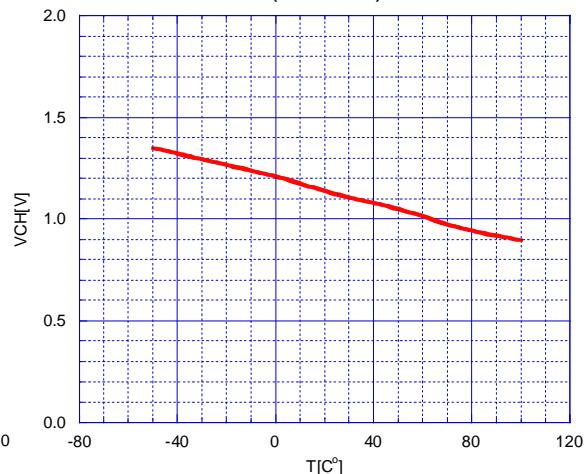
SW Threshold(Low) vs. Temperature
