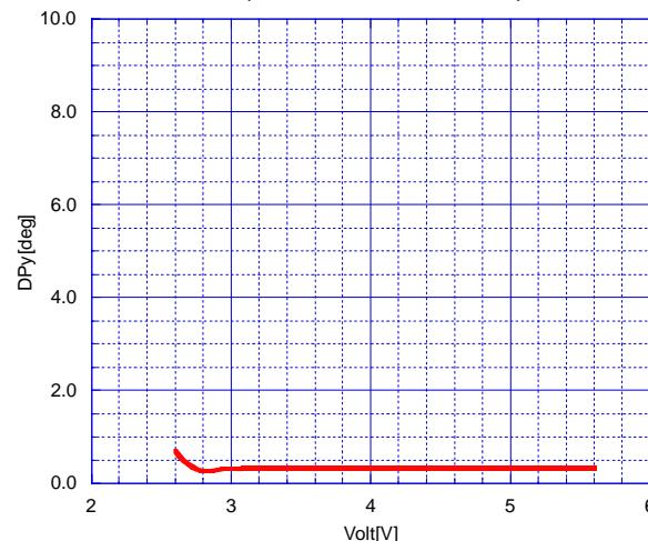
Differential Gain vs. Operating Voltage
