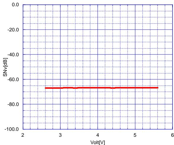
2<sup>nd</sup> Distortion vs. Operating Voltage
