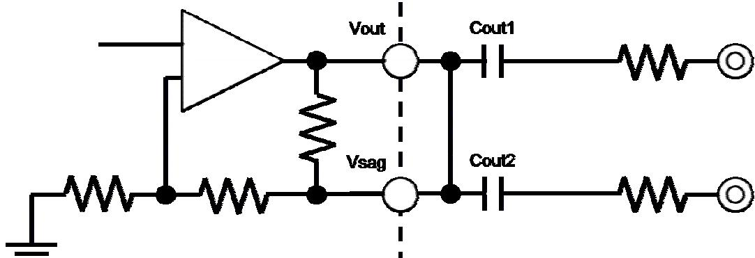
&lt; Using SAG correction circuit &gt;
