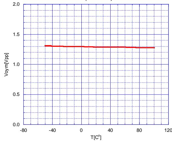
Maximum Output Voltage(Y mode) vs. Temperature
