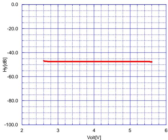
2<sup>nd</sup> Distortion vs. Operating Voltage
