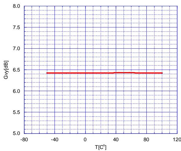
Voltage Gain(C mode) vs. Temperature
