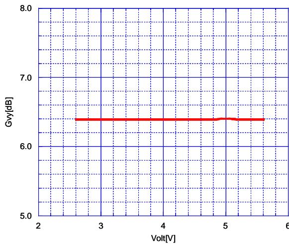
Voltage Gain(C mode) vs. Operating Voltage
