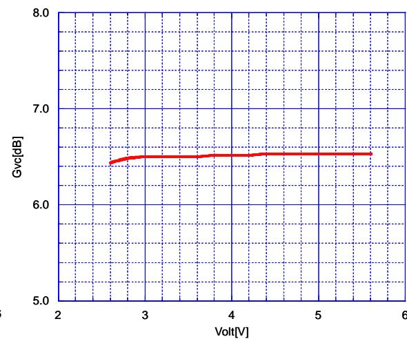
Voltage Gain(V mode) vs. Operating Voltage
