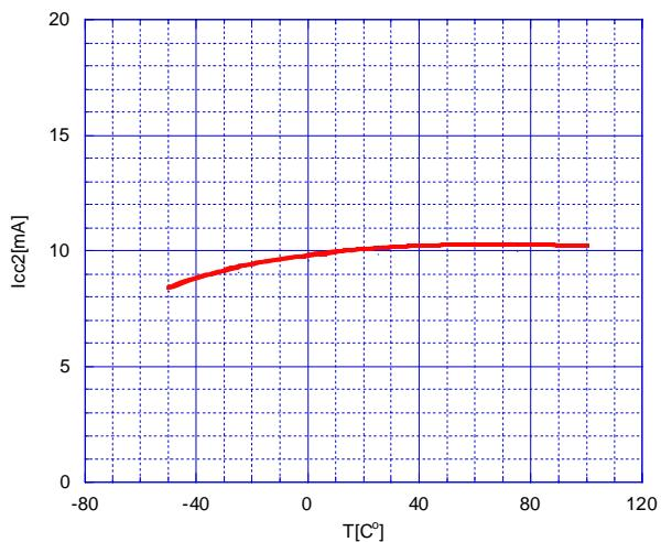
Operating Current1 at Power Save mode vs. Temperature
