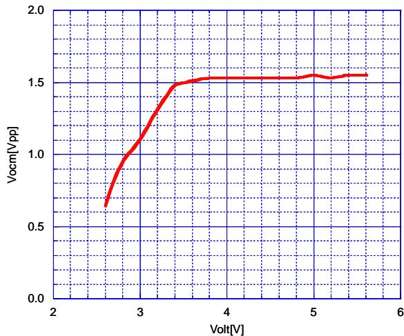
Maximum Output Voltage vs. Operating Voltage
