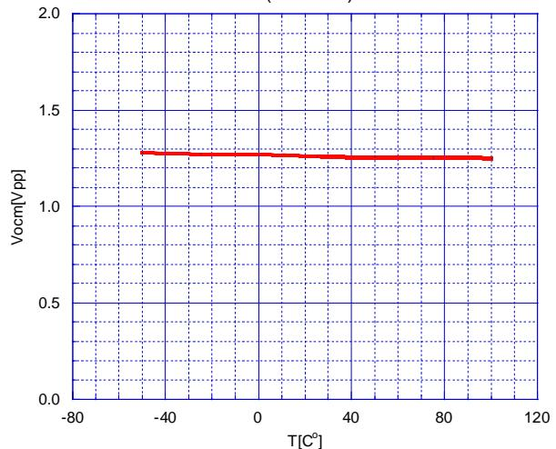
Maximum Output Voltage(V mode) vs. Temperature
