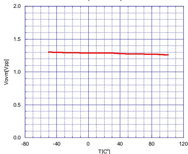
Differential Gain(Y mode)vs. Temperature
