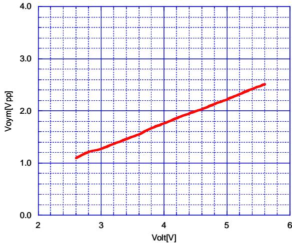
Maximum Output Voltage vs. Operating Voltage
