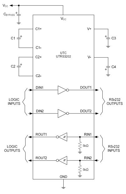
Notes: 1. C3 can be connected to V<sub>CC</sub> or GND.
