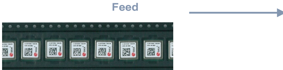
Figure 9: Orientation of NINA-B221 module on tape
