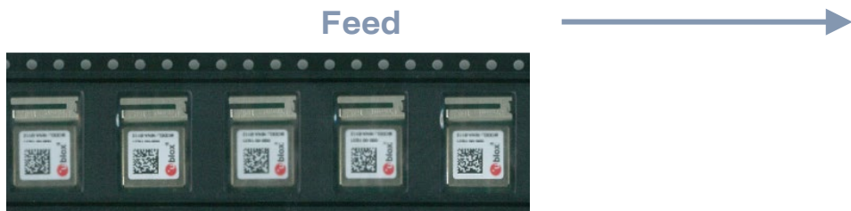
Figure 10: Orientation of NINA-B222 module on tape
