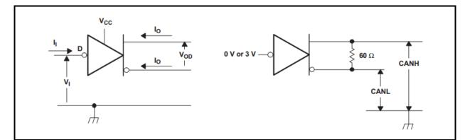
Fig 1 Driver voltage, current and test definition
