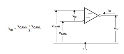
Fig 5 Receiver voltage and current definitions
