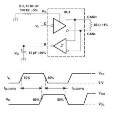
$A_{\text{\tiny $N$}} \ \ \, \text{The input pulse is supplied by a generator having the following characteristics: PRR} \leq 125 \text{kHz}, 50\% \ duty \ cycle, \ t_{\text{\tiny $r$}} \leq 6 \text{ns}, \ t_{\text{\tiny $r$}} \leq 6 \text{ns}.$
