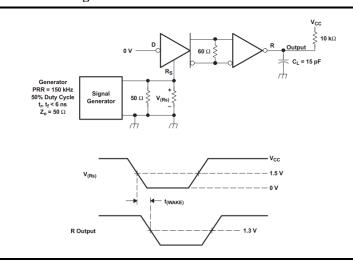
Fig 7 t(WAKE) test circuit and waveform
