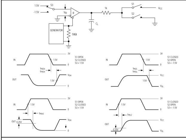
Figure 8 Receiver enable and disable time
