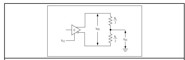
Figure 2 Driver DC test load
