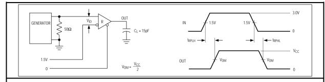
Figure 7 Receiver propagation delay test circuit
