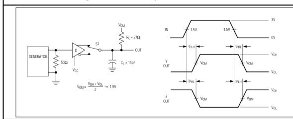
Figure 4 Drive propagation delay
