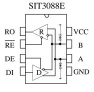
Figure 1 SIT3088E Pin Configuration
