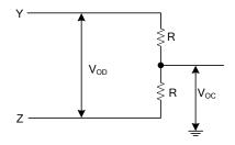
Fig. 1 Driver DC Test Circuit
