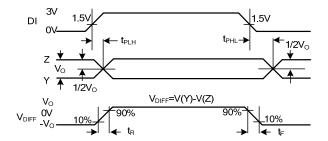
Fig. 5 Driver Propagation Delays
