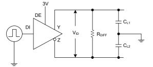
Fig. 3 Driver Timing Test Circuit
