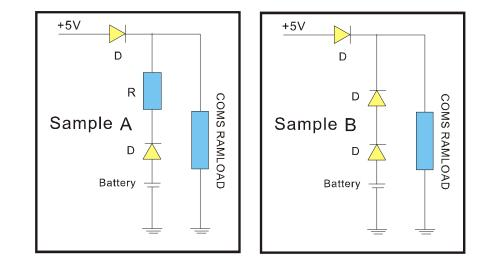
A protection resistor is needed to prevent diode failure from allowing a large current to flow into the battery.
