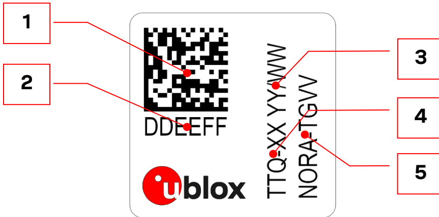
Figure 13: NORA-B1 series module marking
