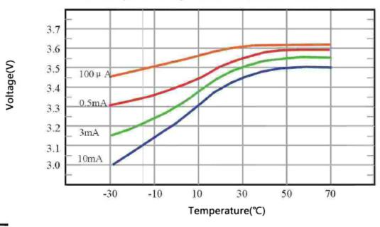
ER10450 Typical Voltage versus Temperature and Current
