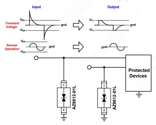
Fig. 1 ESD protection scheme by using AZ9812-01L.
