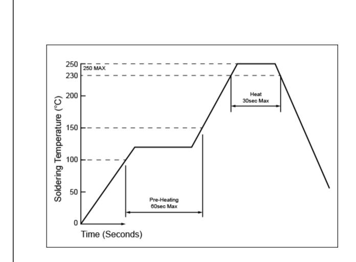
Fig. 1. Recommended Reflow Temp. Profile
