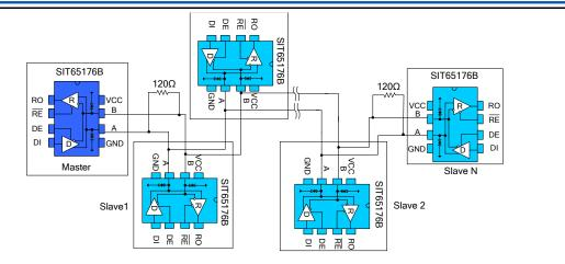
Fig 10 Hand in hand RS485 half-duplex communication network
