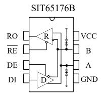
Fig 1 SIT65176B pin configuration
