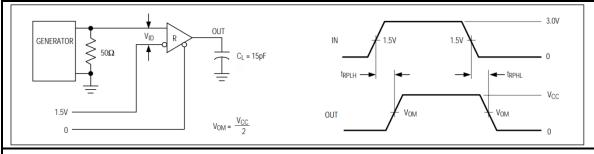
Fig 7 Receiver propagation delay test circuit
