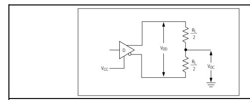
Fig 2 Driver DC test load
