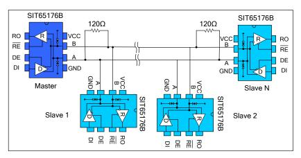
Fig 9 Bus type RS485 half-duplex communication network
