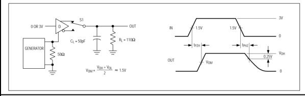
Fig 5 Driver enable and disable time
