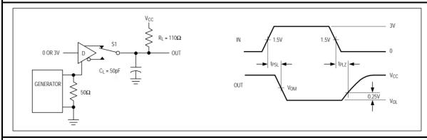
Fig 6 Driver enable and disable time
