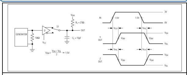
Fig 4 Driver propagation delay
